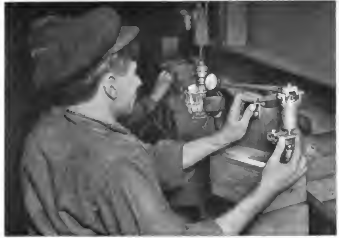
MICROMETER GAUGING THE ROLLERS FOR .002-INCH VARIATIONS.
